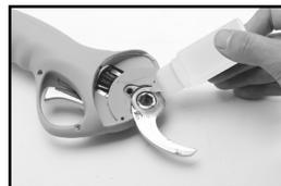
6. When replacing the blades, lubricating oil needs to be added between the blades
