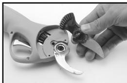
4. Disassemble the pin and remove the moving blade
