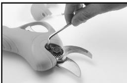
2. Disassemble the screws from the blade nut retaining buckle (this step is critical)
