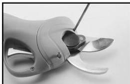
1. Disassemble the screws with a screwdriver and open the lid.
