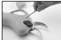
9. Install the nut lock TAB
